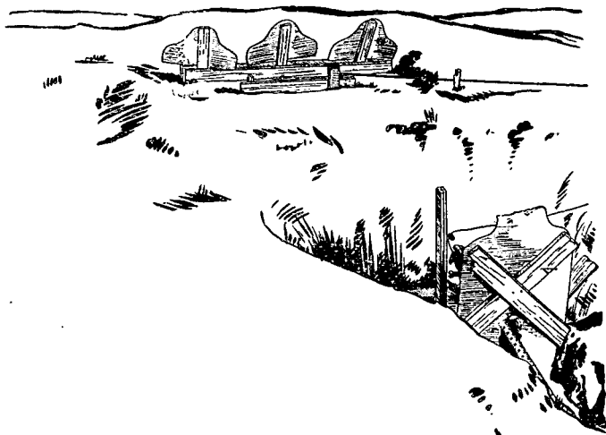
FIGURE 72.—Arrangements for raising surprise targets and producing fire to attract attention. (Cardbord shield protects light machine gun from dirt and dust.)
